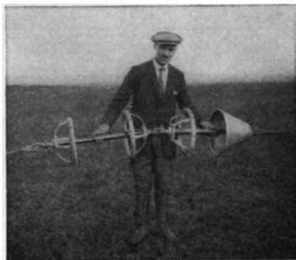
FIG. 1.35. Assembly of two antenna strain insulators in series, both fitted with potential-grading rings and one with a rain shield.
